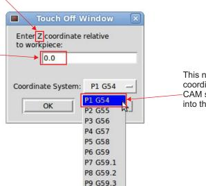
This needs to match the coordinate system that the CAM software is inserting into the q-code.
