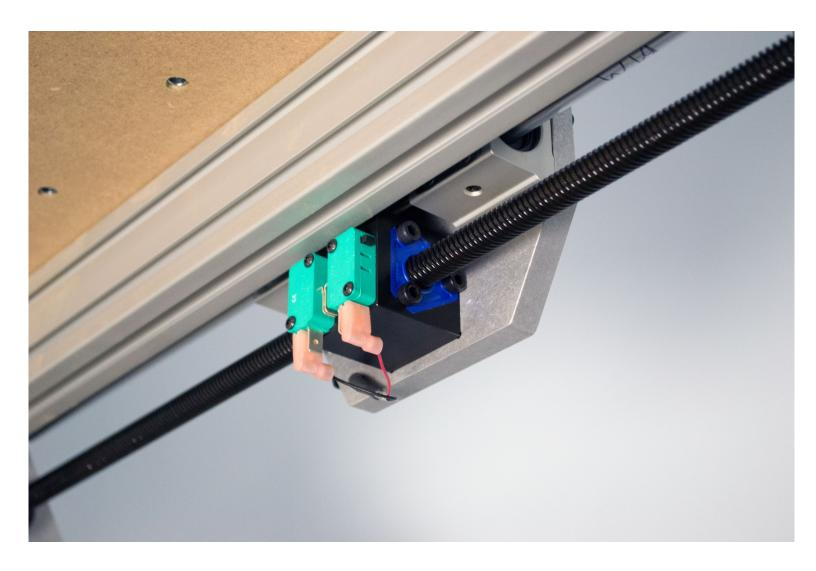
The Y1 and Y2 limit switches have been removed to protect them during transport. Reinstall them as seen above before running the machine.
